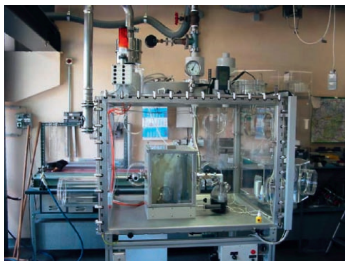
Figure 7: Glove-box for handling of special nuclear material [7].
